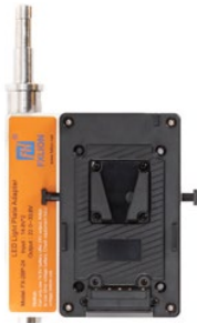
FX-2BP-24 - Plate Adapter Features: 22V-33.6V Output from 2 x 14.8V Batteries Dimension: 206(L)*134.5(W)*45.5(H)mm Weight: 910g
